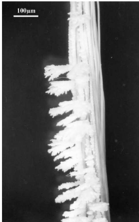
FIG. 7. Deposit processed with homogeneous nucleation ( T > 1300^{\circ}\text{C} ).
